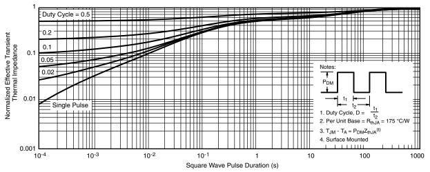
Normalized Thermal Transient Impedance, Junction-to-Ambient
