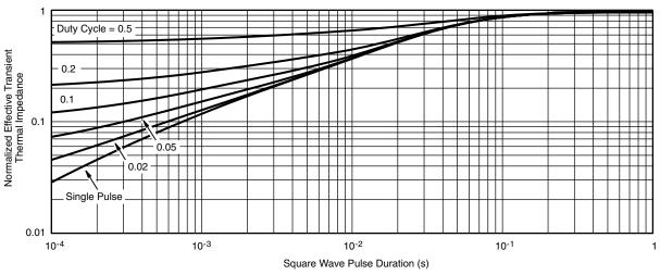
Normalized Thermal Transient Impedance, Junction-to-Foot
