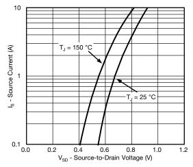
Source-Drain Diode Forward Voltage
