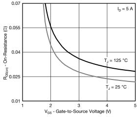
On-Resistance vs. Gate-to-Source Voltage
