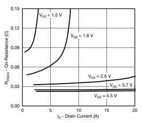
On-Resistance vs. Drain Current and Gate Voltage
