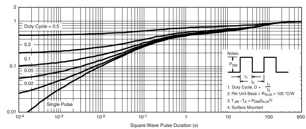
Normalized Thermal Transient Impedance, Junction-to-Ambient
