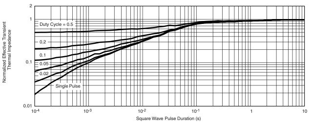
Normalized Thermal Transient Impedance, Junction-to-Foot
