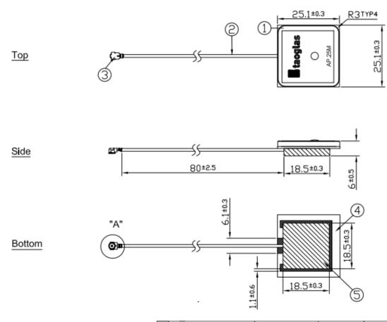
4. The connector orientation has a fixed position to the antenna as per drawing.
