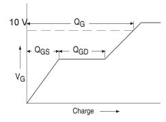
Fig 13a. Basic Gate Charge Waveform
