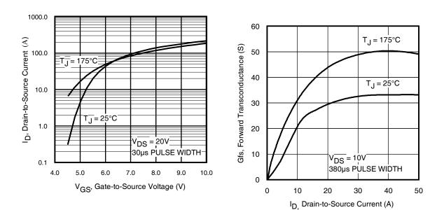
Fig 3. Typical Transfer Characteristics
