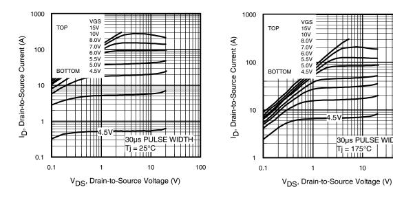
Fig 1. Typical Output Characteristics
