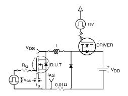
Fig 12a. Unclamped Inductive Test Circuit
