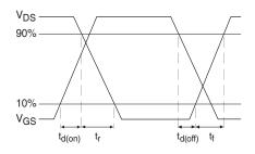
Fig 18b. Switching Time Waveforms
