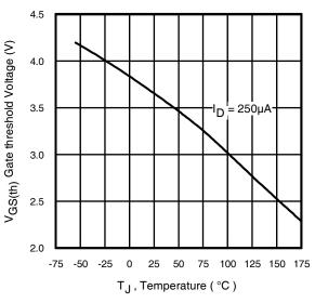
Fig 14. Threshold Voltage Vs. Temperature
