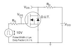
Fig 18a. Switching Time Test Circuit
