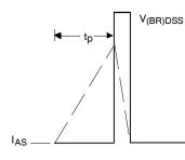
Fig 12b. Unclamped Inductive Waveforms
