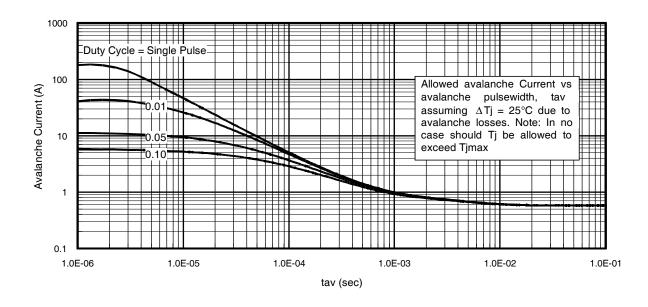
Fig 15. Typical Avalanche Current Vs.Pulsewidth
